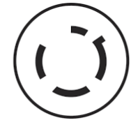
L15-20P NEMA Twist-Lock Plug
